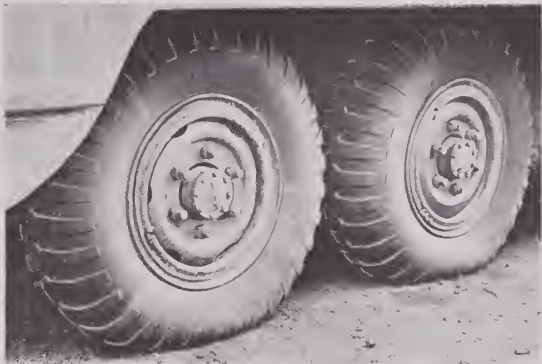
FIGURE 24. 11.00x18 ten-ply desert tread tires used on production DUKW.
